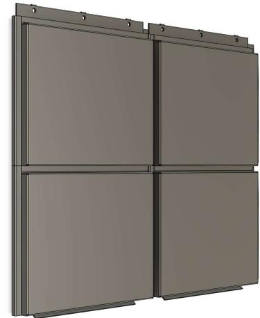
**Material / Patina:** A606-4 weathering steel is a high strength, cold rolled material. A matte finish occurs on the steel from iron oxide. The natural weathering process (patina) will naturally occur after material installation.
